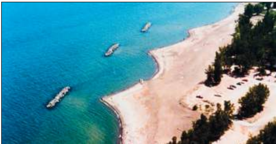
Figure 3-44. Example of littoral sediments being trapped behind offshore breakwaters on Lake Erie, Presque Isle, PA SOURCE: USACE
