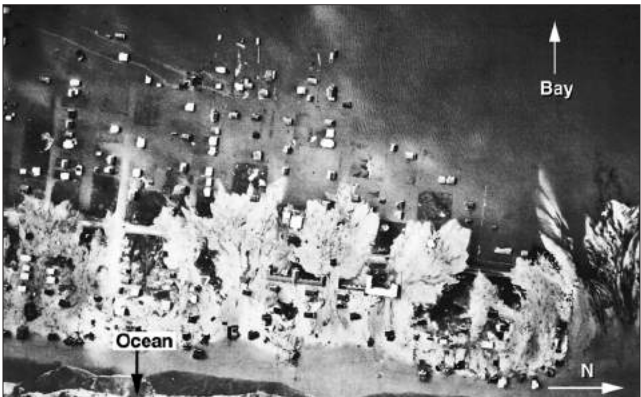
Figure 3-6. Flooding, erosion, and overwash at Fenwick Island, DE, following March 1962 nor'easter
